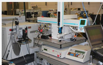
Phosphoproteomics nano-LC platform coupled to a Thermo Scientific LTQ Orbitrap Velos ETD mass spectrometer. Sample flow-path is metal free.
