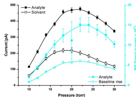
**Figure 3.** Effect of pressure on current and MS signal. Not all the extra current during the analyte plug elution is due to analyte ions: ~17-23% of the TIC increase is due to rise of baseline (see Figure 2). An operating pressure of ~20 Torr ensures optimum ionization with this source geometry.
