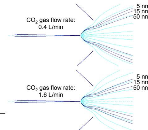
**Figure 7.** The interface model showing the field lines and the trajectories for droplets of 5, 15, and 50 nm. The model was calibrated against experimental data probing the transmission through the conical outlet
