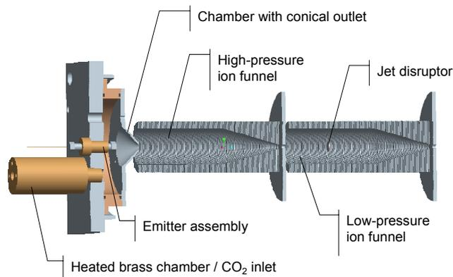
**Figure 1.** The sample is electrosprayed in a chamber with conical outlet maintained at ~20 Torr. CO<sub>2</sub> is heated in a brass chamber and used as sheath gas. A dual ion funnel assembly transfers the ions into the high vacuum region of the mass spectrometer.
