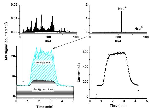
**Figure 2.** Typical solvent (top-left) and analyte (top-right) mass spectra. Total ion current showing a rise in baseline during the analyte plug elution (bottom-left) presumably due to poorly desolvated species (clusters). Current collected on the octopole following the low-pressure ion funnel (bottom-right).
