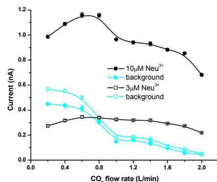
**Figure 5.** Effect of gas flow rate on current. Black traces may suggest concentration-dependent analyte distribution in small and large droplets. Efficiently ionizing analytes prefer small droplets at low concentrations.
