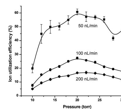
**Figure 6.** Ion utilization efficiency as a function of pressure and liquid flow rate. Reducing the flow rate (implicitly the initial droplet size) has the most dramatic effect on ion utilization efficiency.
