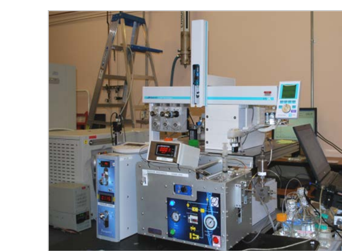
Online Digestion System: Rapid integration of a third party high pressure digestion module (XstreamPCT(tm), Pressure BioSciences Inc.).
